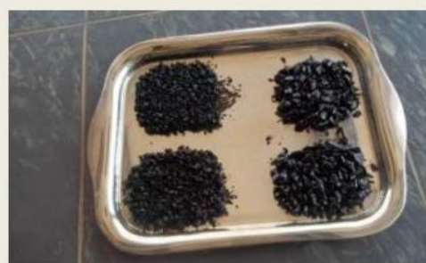
(e) determination of breaking time, coating and setting time
