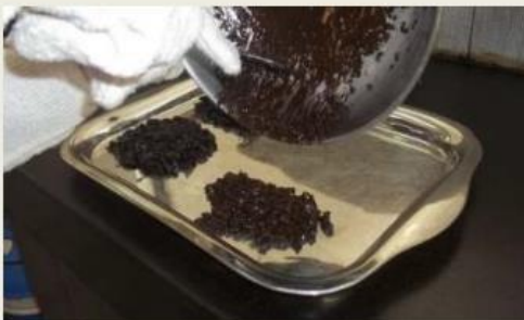
(a) Aggregate form site (b) Required grade of emulsion is added (c) Cold mix is prepared
